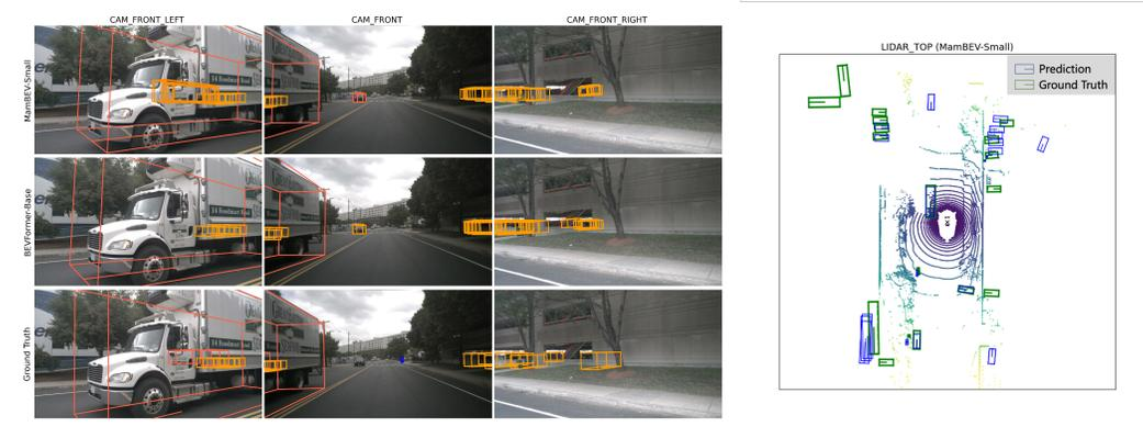
Figure 7: Comparison of MamBEV-Small and BEVFormer-Base on nuScenes val set. We observe that our model can successfully detect objects are missed in the prediction results of BEVFormer-Base.
